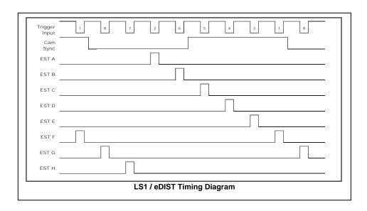
In this LS-1 application, dip switch positions 1-3 should be **OFF** and position 4 should be **ON** configuring the eDist as an 8 coil application. Dip switch position 6 will be set to **OFF** to configure the eDist for the LS-1's hall-effect cam sensor, position 7 will be set to **ON** to configure the eDist for an points type (dwell state low) spark input signal, and position 8 will be set to **OFF** to configure the eDist for the LS-1's falling edge cam sync signal.
